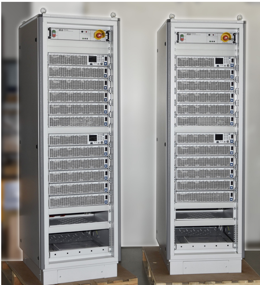
4 PMLA systems with a total of 288 channels
